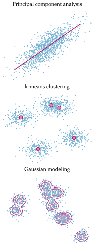
Figure 1.1: Examples of learning tasks: PCA (top), k-means clustering (middle), and density estimation with a Gaussian mixture model (bottom). Data points are represented in blue, and the learned model (the hypothesis) in purplish red.
